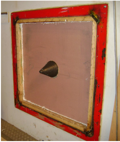
Figure 2.3: Basic Mitt (covering downlight) installation on plasterboard (from source chamber)
