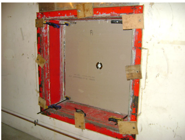
Figure 2.2: Downlight installation in plasterboard (from receiving chamber)
