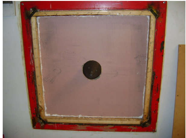
Figure 2.3: Basic Mitt (covering downlight) installation on plasterboard (from source chamber)
