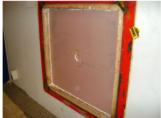
Figure 2.4: 16mm plasterboard fill installation, from receiving and source rooms respectively
